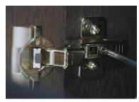
Turn back screw found at the back of the hinge. This can be turned left or right.
