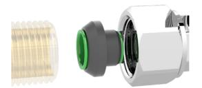
Installation is easy and quick. **Thread** the loose nut connection to the threaded pipe with your hand (no tooling is required), leave it not too tight, ensure that the valve can rotate axially. **Adjusts** the valve in the correct orientation. Once located at your convenience, **tighten** the loose nut preferably using a spanner. Do not over tight the loose nut to avoid cutting the cone washer.
