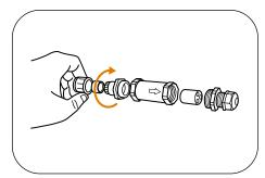
3. Feed the cable through the open mechanism.
