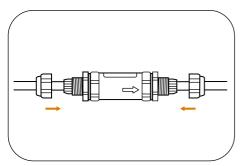
9. Tighten the screw ends.
