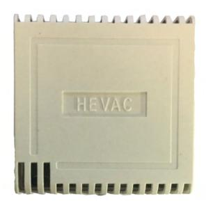
The SRTA-H is an averaging type room sensor to be used in pairs (wired in parallel). It is intended for use with Hevac brand HTC 2 & 4 series controllers. The sensor has a PTC characteristic (increase in temperature = increase in resistance) and changes approximately 28 ohms per degree.
