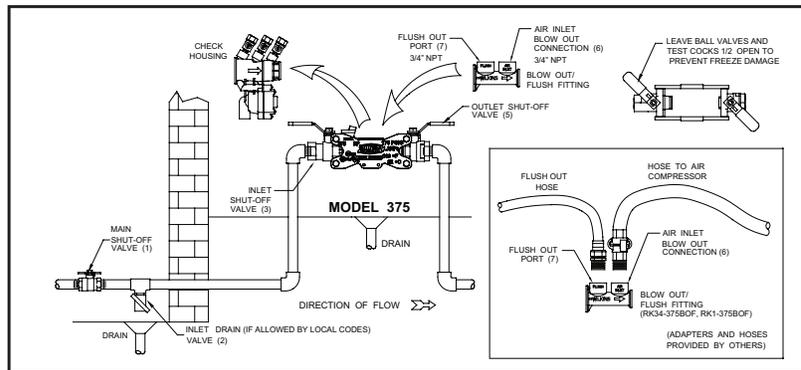
**To blow out system for freeze protection, use the following procedure:**
