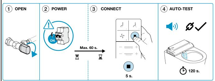
After connecting the power (2), you have 60 seconds to link the remote control.
