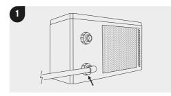
Using the 40mm tail supplied, connect the outlet upstream before any chlorinators, acid injection or other chemical dosing systems.
