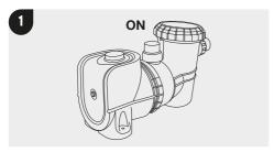
Check there are no water leaks and verify adequate flow to and from the pool.
