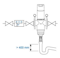
For Multipur AP 65, Multipur AP 80 and Multipur AP 100: Drainage connection min. DN 50
