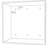
The number of fittings used to fix cabinet will depend on the size of unit, your installer will know the suitable amount depending on the size of your cabinet. Rifco recommends the following minimum;
