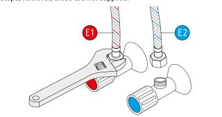
After installation, establish water supply and thoroughly check operation of tapware to ensure that it functions correctly and no water leaks. Plumbers, please ensure a copy of the Installation Instructions are left with the end user for future reference.
