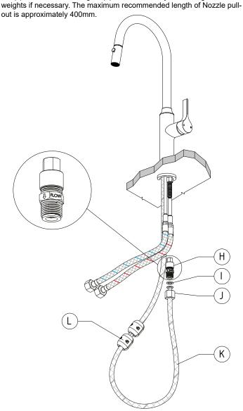
4) Connect the Hot (E1) and Cold (E2) flexible hoses to 1/2" BSP pipework and tighten firmly with a spanner. Ensure hoses do not twist or kink during tightening. Sussex recommends using Stop Cocks/Mini Stops, however, these are not supplied.
