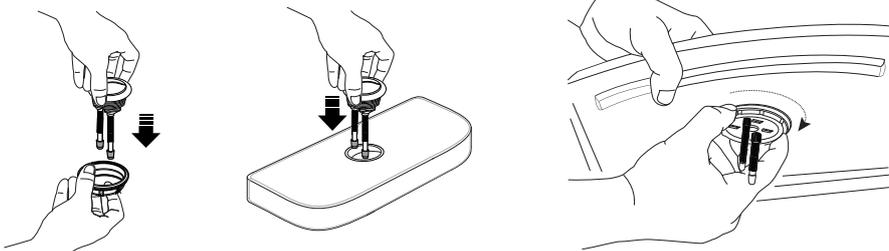
Ensure button rods are aligned with full & 1/2 flush on outlet valve.
