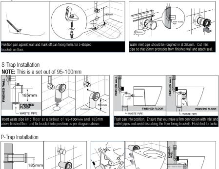
Push pan back into position. Ensure that you make a firm connection with inlet and outlet pipes and avoid disturbing the floor fixing brackets. Flush test for leaks.
