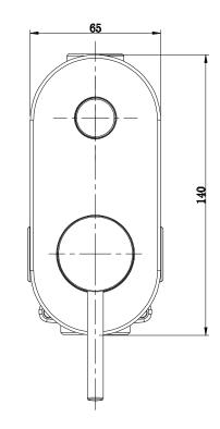
2-Rp1/2 2-Rp1/2 Rp3/4 65mm - 75mm install depth
