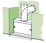
When installing the hood in ducting version, a rigid or a flexible pipe with the diameter corresponding to the flange diameter is used in order to connect the hood to the air outlet piping.
