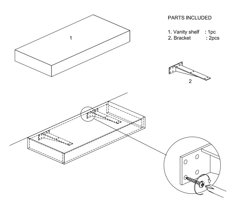
Brackets must be fixed to a solid wall or timber noggins with appropriate fastenings (not supplied).
