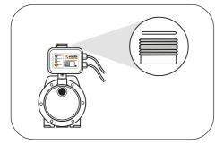
Hold the Mechanical Switching Unit (VFB-MSU25) over the outlet and connect the loose nut. Do not overtighten. The rubber washer will lock this in place.
