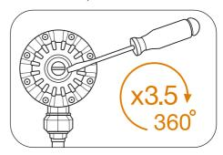
Confirm the pressure has been correctly adjusted by slowly opening a tap outlet and checking the gauge on the side of the VFB-APC. If the gauge reads 2.2, the cut-in pressure has been successfully adjusted.
