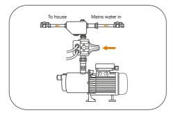
Using a flat head screwdriver, turn the adjustment screw clockwise until you reach the correct pressure (approx 3.5 full 360° turns).
