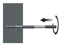
Screw a fixing bolt into each fixing plug using a 8 mm spanner until the spanner contacts the wall
