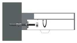
Screw a metal nut onto each fixing bolt to secure the basin. Caution: Do not over -tighten, as this may damage the materials.
