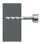
Drill two holes in the required position on the wall using a 14mm masonry drill bit, to a depth of 75mm
