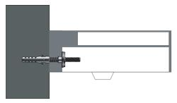
4. Place the basin in position against the wall, iocating the fixing bolts through the holes in the rear of the basin. Push a plastic washer, followed by a metal washer, onto each fixing balt.
