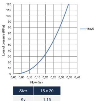
Kv (m3/h), cubic meters per hour that flow through the valve generating a loss of pressure of 1 bar.
