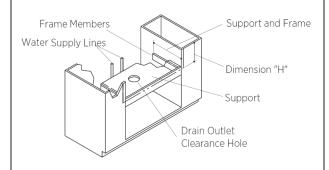
6. Apply some approved flexible watertight silicone to the top of the sink. DO NOT USE EPOXY OR ANY OTHER SOLID ADHESIVE AS THIS MAY CRACK THE SINK OVERTIME AND WILL VOID THE WARRANTY, then place the benchtop over the top of the sink. wipe away excess silicone, and leave to cure for 24 hours before use
