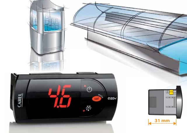
**easy compact** is the ideal solution for applications where the space available for housing the controller is limited: the depth occupied internally is just **31 mm**, while still featuring **2 Hp** relay outputs for the control of refrigeration compressors without requiring additional intermediate relays.
