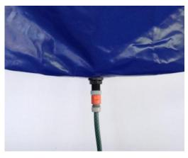
Connect drain hose from the cassette cleaning bag outlet to a 20 litre drum or container for waste water.
