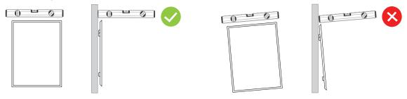
5. Hook mirror to the wall mounted bracket, you can also use silicone to mount the mirror permanently.
