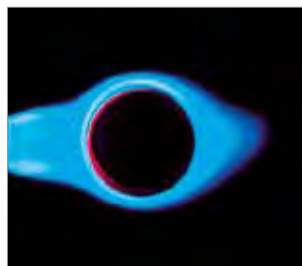
High flame temperature based on cyclone swirl
