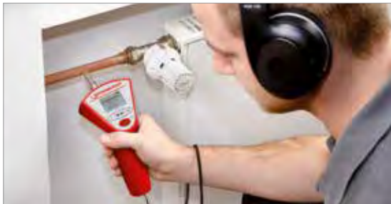
Acoustic leak detection of heating installations
