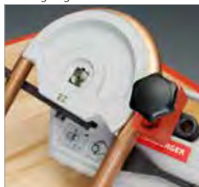
Forged aluminium segments with bending angle scale
