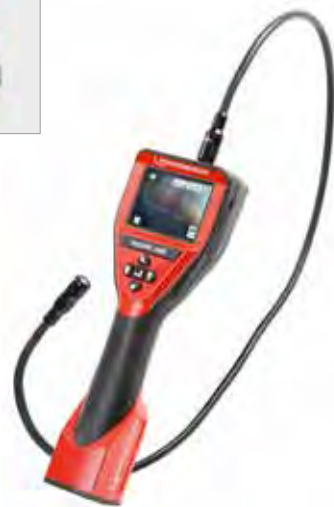
Camera head with high-performance LEDs
