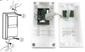
Remove the faceplates (1 and 2) and unscrew the screws to open the control
