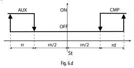
Reverse operation (r3 = 2), in the case of 1 compressor output (CMP)
