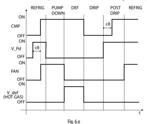
Key <u>CM</u>P Refrig Compressor Cooling V\_Pd Pump down valve Pump down Pump down stage FAN Evaporator fan Defrost V\_def Hot gas valve Drip Dripping Post drip Post-dripping Evaporator Condenser Defrost probe V2 Thermostatic expansion valve Liquid receiver Filter-drier Liquid gauge Time
