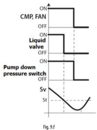
Note: as the pressure switch is connected to terminals 101-102, do not enable pump down on Smartcella 3PH (check that c7=0, H1≠5).
