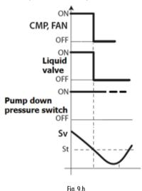
Note: do not enable pump down on Smartcella 3PH (check that c7=0, H1≠5).
