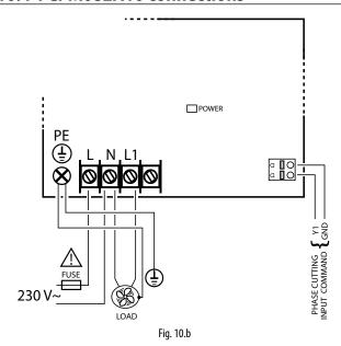
Warning: The earth-protection is connected to the case through the fixing screws
