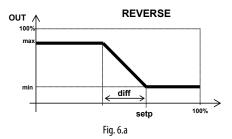
All the functions and observations applied in Direct mode, are valid symmetrically in Reverse mode. Direct mode is set by default (alternatively the selection can be associated with dipswitch 4).and by digital input. The values of the set point, differential, minimum and maximum output can be set by dipswitch or by setting the parameters. If the minimum output set is greater than the maximum output, the value is limited internally to maximum output.
