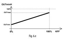
The function is enabled when probe B3 is enabled. By default probe B3 is disabled and consequently so is the function.
