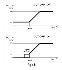
The change from the minimum output to zero output and vice-versa is performed using an hysteresis, so as to avoid unwanted fluctuations. The hysteresis can be set by parameter (default 2% of the operating range of the probes)
