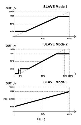
Normally the control signal is supplied by an external controller using the 0/10V standard, however any signal compatible with those allowed for probe input B1 can be used, setting the input accordingly.
