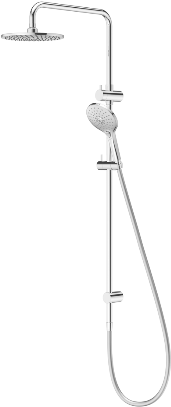
●●●● Domaine 3 Function Twin Rail Shower WELS 3 star, 9L/min 1155mm rail 220mm overhead shower Strong and durable 1.5m hose 3 function hand shower Easy retrofit installation
