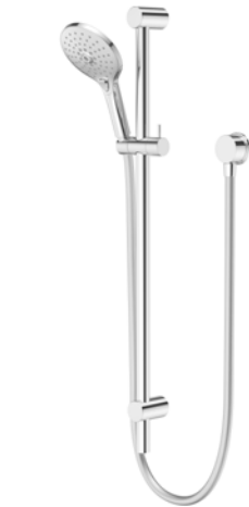
●●●● Domaine 3 Function Brass Rail Shower WELS 4 star, 7.5L/min 655mm rail Strong and durable 1.5m hose Easy retrofit installation
