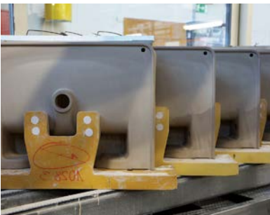
PRODUCTION OF SAPHIRKERAMIK WITH THE CASTING TECHNOLOGY INVENTED BY LAUFEN
