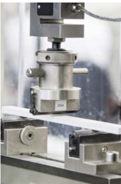
SAPHIRKERAMIK HAS A TWO TO THREE TIMES HIGHER BENDING RESISTANCE THAN TRADITIONAL CERAMICS
