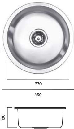
Solus Round Sink 304 grade stainless steel Sound deadening pads under bowl 430mm 0 taphole Sink packs also available with matching wire basket and chopping board Suitable for inset or undermount installation
